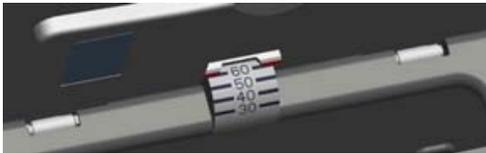
When you are positioning the antenna during the Antenna Pointing process, the protractor provides the current angle of the antenna so that you can adjust it to the Antenna Angle specified on the pointing screen.
