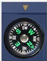
Reference the compass during the Antenna Pointing process to get the correct Compass Direction needed for the antenna. The illustration shows an example of a South-West orientation.
