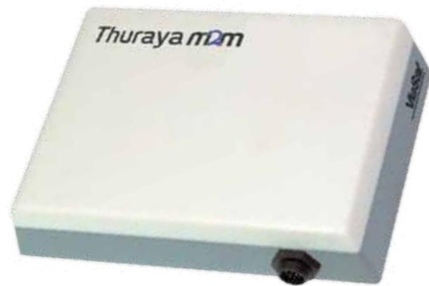
The FT2225 satellite M2M terminal enables connectivity for remote assets and sensors for monitoring, control and security of critical applications in the oil and gas, utilities, mining, banking and government sectors.
