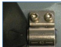
elevation angle correctly set, place the Thuraya IP+ on a flat surface with the antenna facing in the direction of the satellite as determined in step 3.
