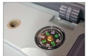
location will be highlighted in green. With the **ThurayaIP** terminal upside down, use the integrated compass to determine the direction of the recommended satellite. You must be able to obtain a clear view of the satellite in the sky for the **ThurayaIP** to connect to the network. If the recommended satellite is obstructed from your location, consider using the alternate satellite instead. If neither satellite is
