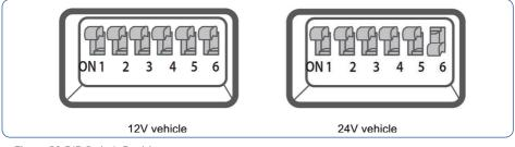
Figure 21 DIP Switch Position
