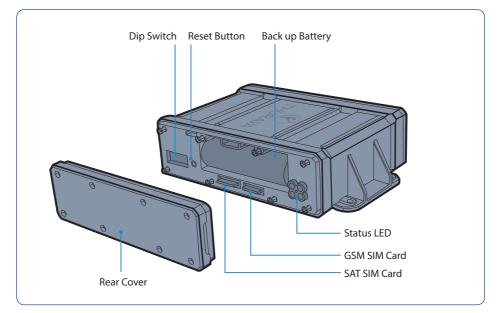
Figure 5 T2M-DUAL 1 Terminal Rear Side
