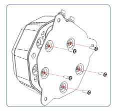
Figure 18 Antenna Bracket Fixing
