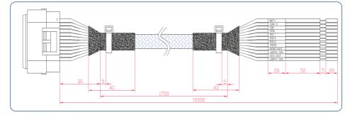
Figure 10 Cable Assembly Drawing
