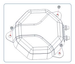
Figure 19 Antenna Fixing
