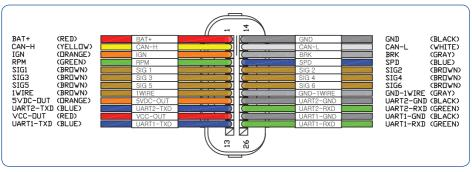
Figure 11 Connector Pin Allocation
