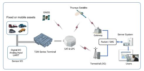
Figure 1 T2M-DUAL System Diagram
