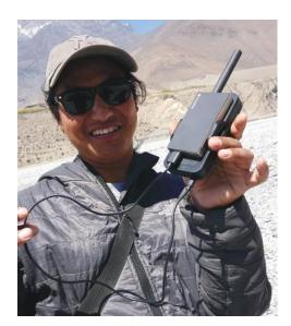
Bluetooth connection between the devices and the WiCis-Sports app on a smartphone (the app is the interface that gathers health data and allows it to be transmitted in usable form over the internet). Finally, the smartphone was connected to the Thuraya SatSleeve+ to establish a continuous data stream via satellite.
