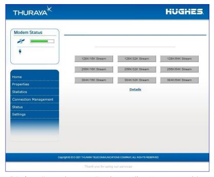
Accessible from the Main Menu, the Connection Management Screen allows you to select from nine Quality of Service (QoS) quick connect buttons. Each button can be customized using the Details link on the Connection Management Screen. The customization parameters for each button are as follows:
