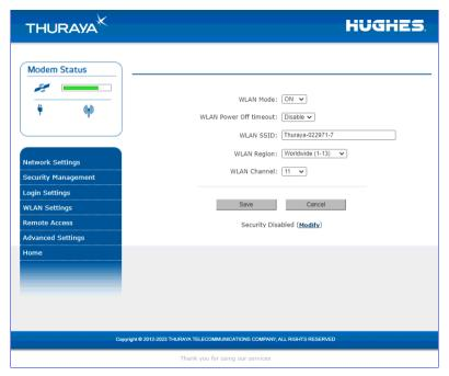
The **WLAN Configuration Screen** allows you to configure the integrated WLAN Access Point (AP) which can support up to eight simultaneous clients using 802.11b/g/n.
