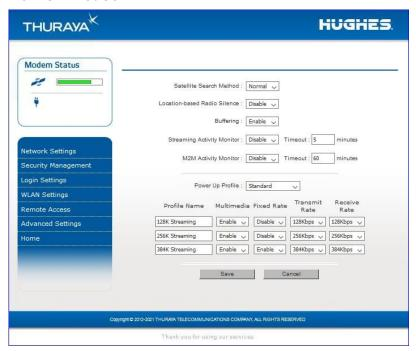
The **Advanced Settings Screen** allows you to modify several key operating parameters in the unit.
