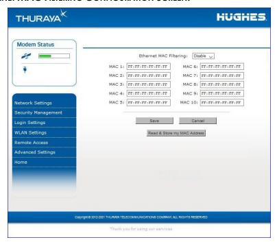
From this screen you can enable and disable Ethernet MAC filtering and you can specify up to eight MAC addresses in the white list. Any changes to this configuration screen will be effective upon a restart of the UT.
