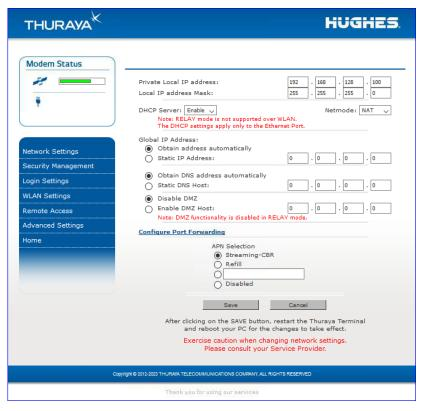
After executing the necessary First Time Set-up steps to configure the Thuraya IP Voyager, you may want to select the **Network Settings Screen** to check your network configuration. This screen provides you with control over key network access parameters. Here you find the appropriate Domain Name Service (DNS) and the Access Point Name (APN) information configured by your Service Provider. You are also given the ability to make changes.
