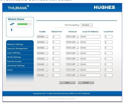
Note that a new PDP context is required for Port Forwarding changes to take effect. Port Forwarding is not compatible with Relay Mode and is disabled automatically when Relay Mode is enabled.
