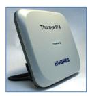
much like commercially available wireless routers. Note that the Wi-Fi Access Point in the Thuraya IP+ uses a separate subnet and DHCP server than the wired Ethernet port. An internal router allows IP traffic to flow seamlessly between the two subnets and out over the satellite link.
