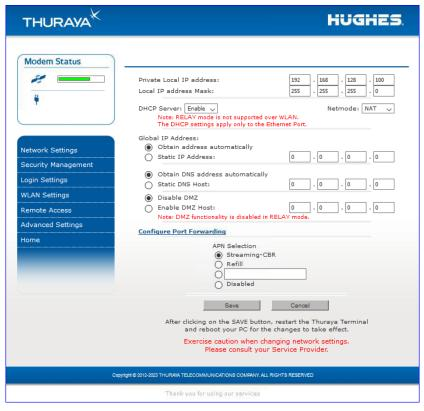
After executing the necessary First Time Set-up steps to configure the Thuraya Orion IP, you may want to select the **Network Settings Screen** to check your network configuration. This screen provides you with control over key network access parameters. Here you find the appropriate Domain Name Service (DNS) and the Access Point Name (APN) information configured by your Service Provider. You are also given the ability to make changes.
