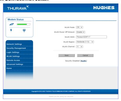
The **WLAN Configuration Screen** allows you to configure the integrated WLAN Access Point (AP) which can support up to eight simultaneous clients using 802.11b/g/n.
