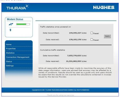
The **Statistics Screen** provides you with an estimate of your data usage. Data usage figures are obtained by counting the bytes in the IP packets
