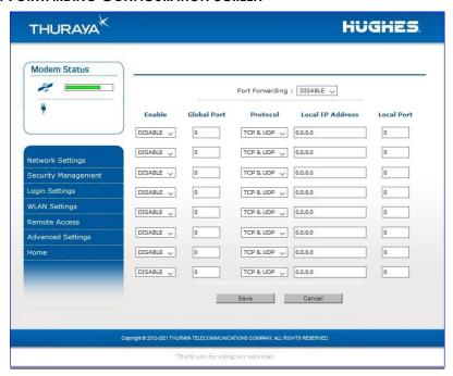
Note that a new PDP context is required for Port Forwarding changes to take effect. Port Forwarding is not compatible with Relay Mode and is disabled automatically when Relay Mode is enabled.
