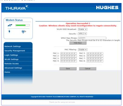
The **WLAN Security Screen** allows you to configure WLAN security parameters, including enabling/disabling Wired Equivalent Privacy (WEP), hiding the SSID and setting Media Access Control (MAC) filters.
